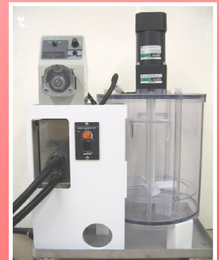
Slurry Tank, Pump, and Flow Controller
